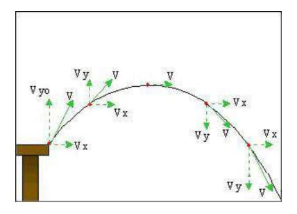
The projectile has a constant horizontal velocity and a vertical velocity that changes uniformly under the influence of the acceleration due to gravity.
