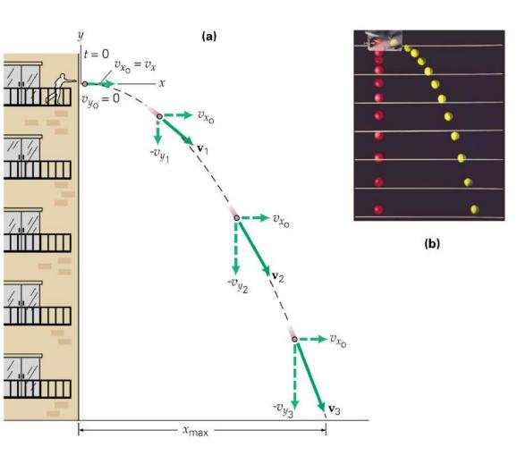
In the figure we can see that the vertical velocity and position increase with time as those of a free-falling body. Note that the horizontal distance increases linearly with time, indicating a constant horizontal velocity.
