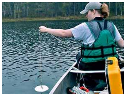
Citizen volunteers use Secchi disks to collect data on water clarity.
