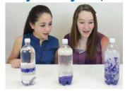
When the 1L bottle is shaken, blue and white beads mix as expected. However, when allowed to settle, the beads separate, white at the top and blue at the bottom. Then, the two separated colored beads slowly come together in the center of the liquid. How often do you see something floating in the middle of the liquid? Great for illustrating so many concepts: solubility, density, miscibility, the salting out effect and more.
