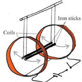
coils produces an almost uniform magnetic field in the space where the iron rods are hanging.
