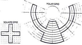
On the polar grid, lines which are to appear vertical become parts of radii. Lines which are to appear horizontal become arcs of circles.
