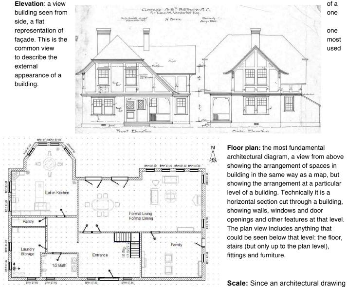
must fit on a piece of paper, you must scale down the actual dimensions of the building when you draw the blueprint. For example, if the height of your building is 12", but you need to fit it within an 8" space on your paper, you would use a scale of 2:3. This means that every 2" on your page actually represents 3" of your actual building. The scale is typically expressed as a ratio (e.g. 2:3) or as a fraction (e.g. 2/3), and should be displayed on your page.
