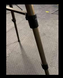
Tripod Joints - Open the latch and extend the leg to however long you need the tripod to be. Make sure to securely close it to make sure the tripod doesn't slide down during the shoot!
