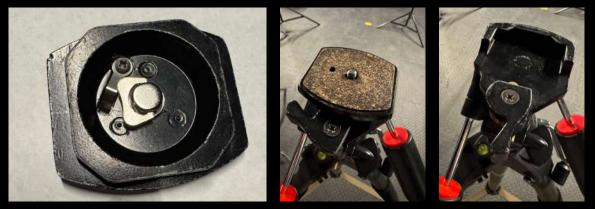
Quick Release Plate - This is what you attach to the bottom of the camera. Make sure to secure it tightly so the camera doesn't move on the tripod, but don't overdo it!
