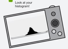
You will usually want to see a bell shaped histogram that is slightly to the right of center. This makes post production easier as bringing a slightly over-exposed image down doesn't introduce noise whereas increasing exposure in post on an under-exposed image will.
