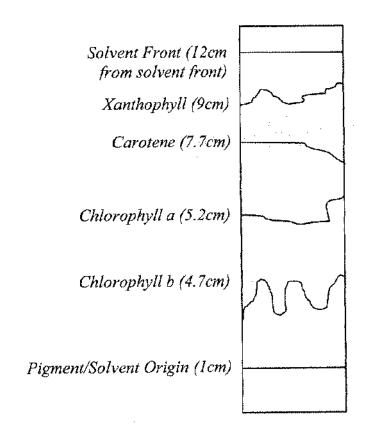
R<sub>f</sub> = <u>distance moved by pigment from original spot</u> distance moved by solvent from original spot
