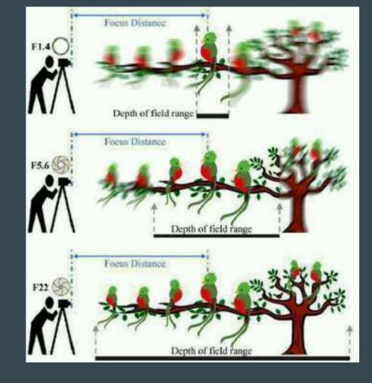
How a real camera does Shallow Depth of Field
