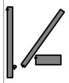
10. The cable is connected 10.0 m from the hinge, and makes an angle of 60.0° with the 12.0 m long, 8.00 kg beam. The sign hangs 3.10 m from the hinge. Find the tension in the vertical cable, and the horizontal and vertical components of the force exerted by the wall. Be sure to give the direction of the components.
