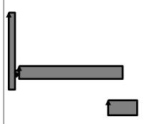
8. The cable makes an angle of 25.0° with the 16.0 m long beam. The sign hangs 5.20 m from the left side of the beam. Find the tension in the cable, and the horizontal and vertical components of the force exerted by the wall. Be sure to give the direction of the components.
