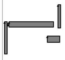
12. The rod is connected 3.20 m from the left side of, and makes an angle of 38.0° with the 4.00 m long beam. The box is centered 1.20 m from the left side. Find the force along the rod, and the horizontal and vertical components of the force exerted by the wall. Be sure to give the direction of the components.
