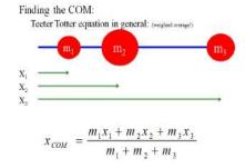
Example: Find the distance the COM is from the left side of the beam. The 45.0 kg uniform beam is 14.0 m long, has a 12.0 kg box 4.0 m from the left side, and a 30.0 kg box centered 13.0 m from the left side.
