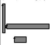
9. The horizontal cable is connected 4.70 m from the hinge, and makes an angle of 54.0° with the 5.00 m long, 5.30 kg beam. The sign hangs 3.00 m from the hinge. Find the tension in the cable, and the horizontal and vertical components of the force exerted by the wall. Be sure to give the direction of the components.
