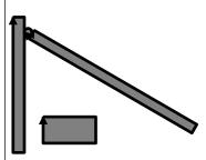
11. The cable is connected 1.50 m from the left side, and makes an angle of 48.0° with the 2.00 m long beam. Find the tension in the cable, and the horizontal and vertical components of the force exerted by the wall. Be sure to give the direction of the components.
