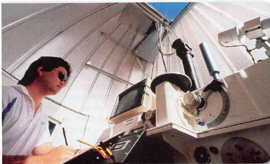
■ Figure 15 This UV-visible spectrometer (UV-Vis) is used to measure ozone and other stratospheric gases during the dark winter months in Antarctica.
