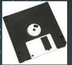
Floppy disks were used in the early days of computing but are rarely seen today. Floppy disks were a way of saving your computer files. The thumb drive and CD-RW's replaced floppy discs as preferred methods of saving electronic files, and it is difficult to find computers with built-in floppy disk readers nowadays.
