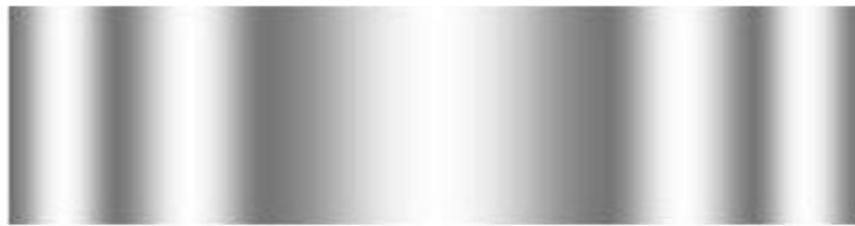
Screen pattern after light diffracts through a single slit (bright center)
