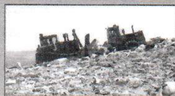
A bulldozer and compactor compact waste at a landfill.
