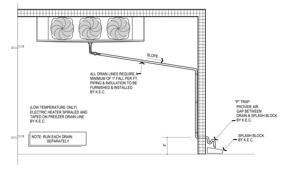
**EVAPORATOR COIL DRAIN DETAIL** SCALE: NTS.
