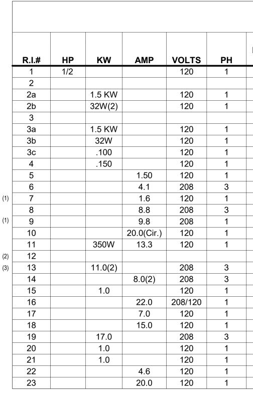
(1) SEE SHEET ??? FOR EXACT LOCATION. ITEM FURNISHED W/MAIN-FUSED DISCONNECT SWITCH. (2) EXTEND CONDUIT DOWN FROM JUNCTION BOX MOUNTED ABOVE FINISH CEILING TO CONTROL PANEL BY E.C. SEE SHEET K-502 & K-503 FOR FURTHER VENTILATOR DETAILS. (3) EXTEND 1/2" DIA. OPEN RIGID CONDUIT FROM TOP OF PULL BOX UP IN WALL TO 6" ABOVE FINISH CLG. BY E.C.
