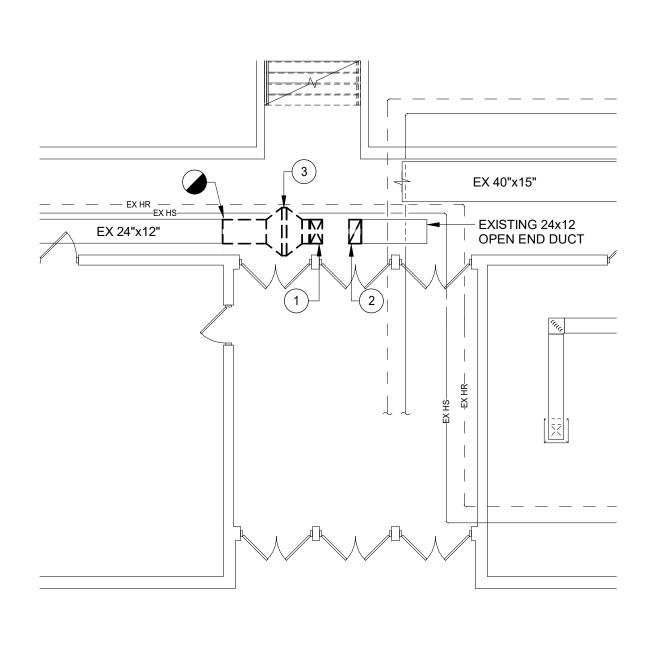
PARTIAL FLOOR PLAN - DEMOLITION - RTU-6
