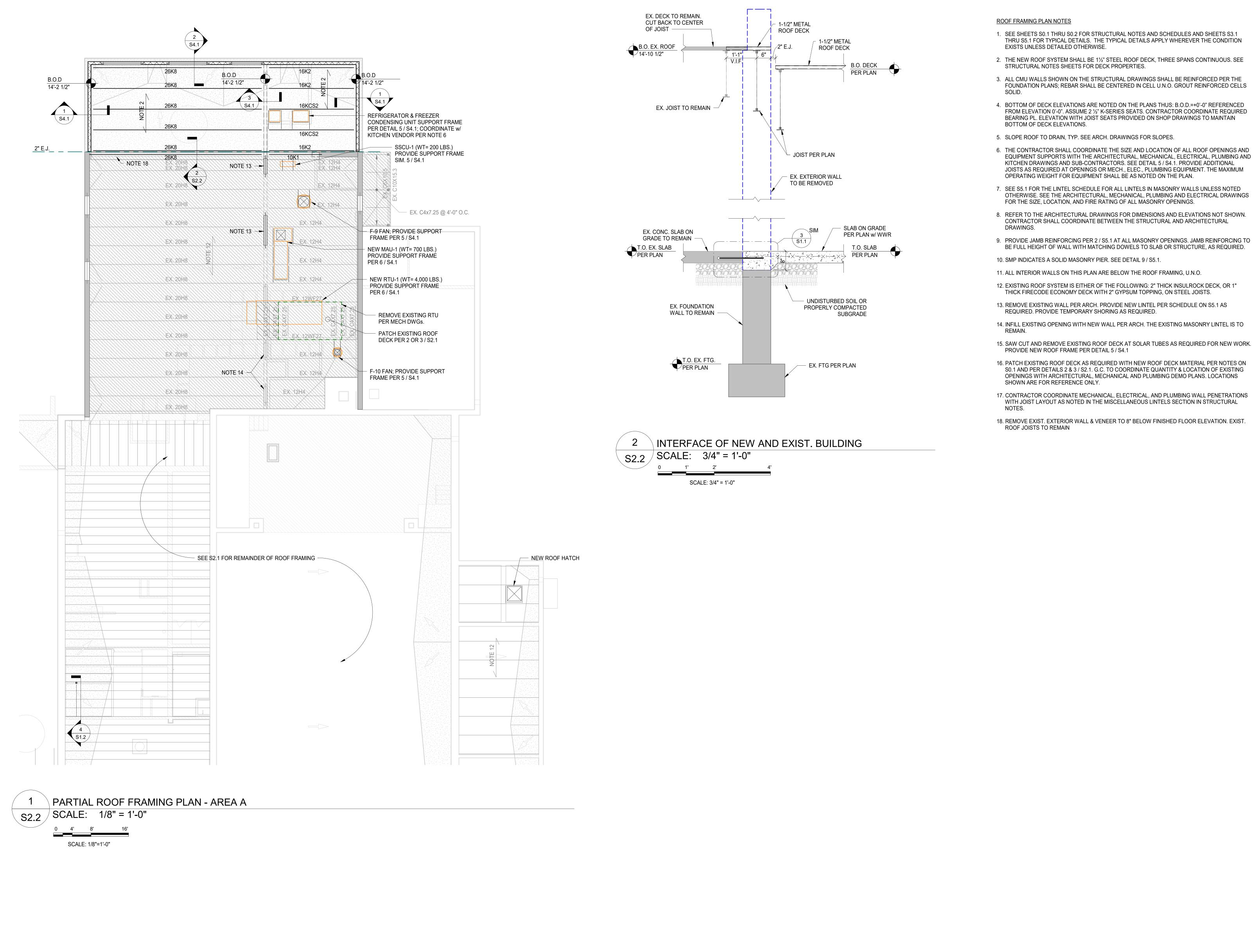
18. REMOVE EXIST. EXTERIOR WALL & VENEER TO 8" BELOW FINISHED FLOOR ELEVATION. EXIST.
