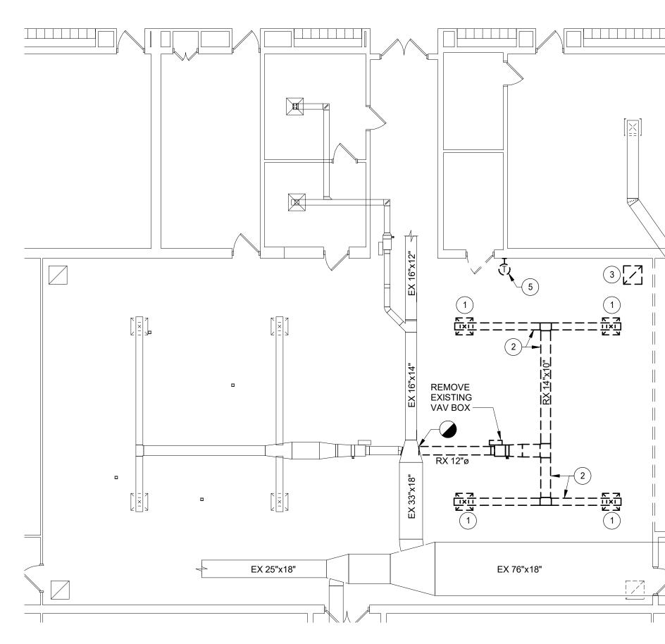
PARTIAL FLOOR PLAN - MEDIA CENTER - DEMOLITION - ALT. GC-2 1/8" = 1'-0"
