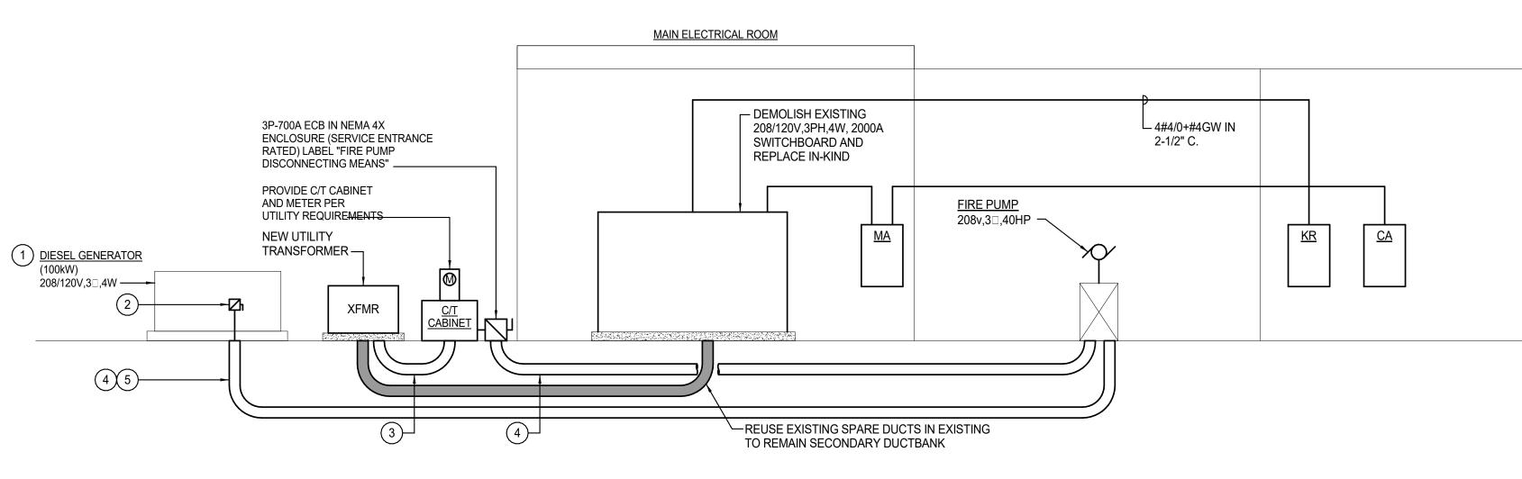
SCHEMATIC POWER RISER DIAGRAM SCALE:NONE
