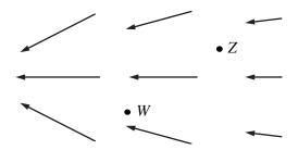
The figure above represents an electric field created by charged objects that are not shown. The field vectors and the locations W and Z are in the plane of the page.
