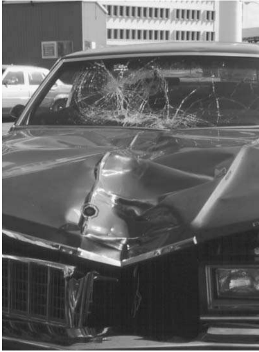
Figure 9.17 Typical pattern of damage to motor vehicle that has impacted a pedestrian. Dented hood and impact site on windshield.
