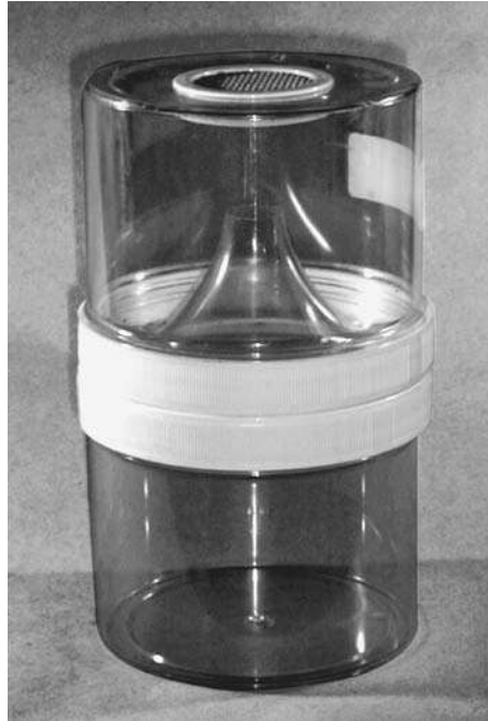
Figure 4.9 A commercially available rearing container that can be used for rearing terrestrial flying and some aquatic flying insects. The container is fitted with a cone that directs newly emerged adults into the vented top portion where they are held until the container is emptied. (Photo courtesy of Jason H. Byrd.)
