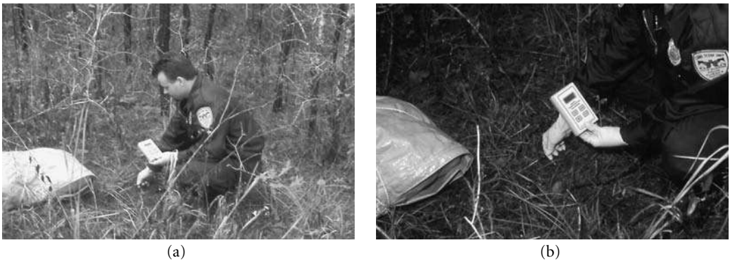
Figure 3.5 (a) Ground surface temperature should be recorded from the top surface of bare soil or any ground cover present (i.e., leaves). (b) Soil temperature also should be recorded at a depth of 10 and 20 cm, at a distance of 15 to 20 cm away from the remains. (Photos courtesy of James L. Castner.)
