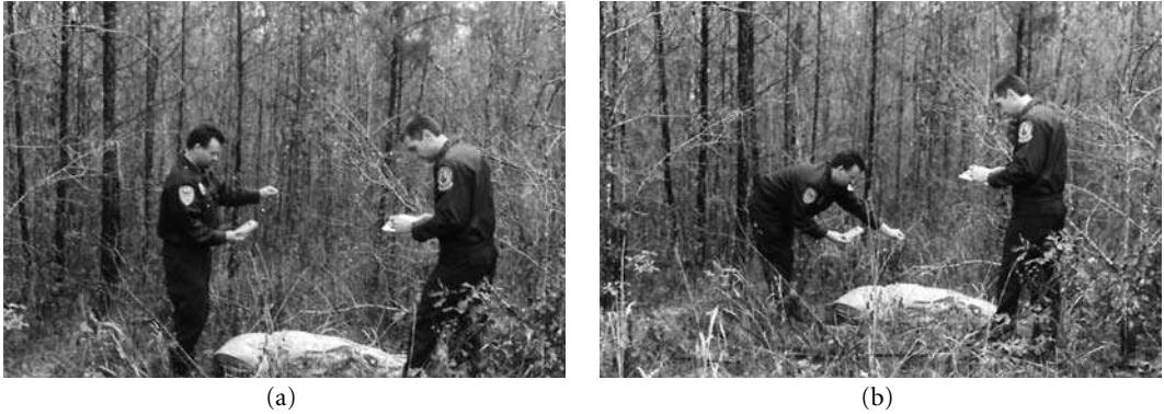
Figure 3.4 (a) Ambient air temperature should be recorded at a height of approximately 4 ft (1.3 m) above (or in close proximity to) the remains. This temperature reading will be used to correlate scene temperatures with National Weather Service observations. (b) An ambient air temperature reading should also be recorded at a height of 1 ft (0.3 m) above (or in close proximity to) the remains. This temperature reading will allow the forensic entomologist to determine the occurrence and effect of microclimatic conditions at the scene. (Photos courtesy of Jason H. Byrd.)
