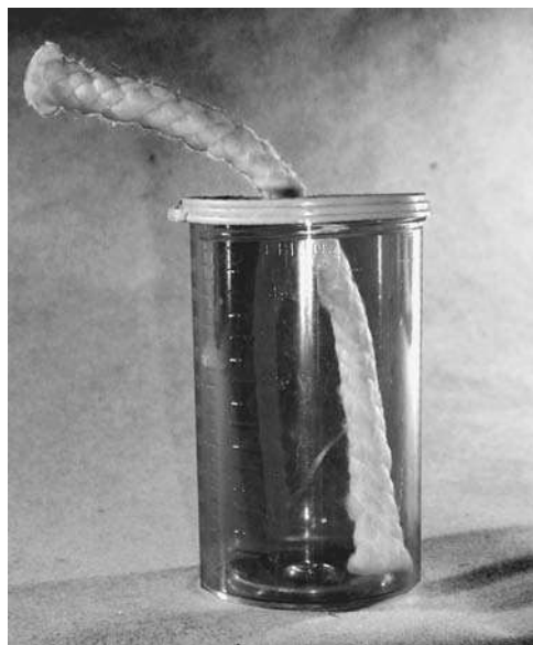
Figure 4.12 In laboratory rearing colonies, an open cup of water can cause many flies to drown, eventually possibly decimating the colony population. A small specimen container, with a dental wick inserted through a hole in the lid works well as a constant source of fresh water for the fly colony. (Photo courtesy of Jason H. Byrd.)
