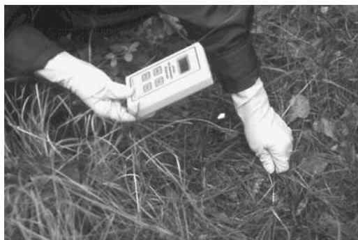
Figure 3.10 It is important to record soil temperatures at a point 3 to 6 ft (1 to 3 m) from the body. These should be recorded from under any ground cover at a depth of 4 in. (10 cm) and 8 in. (20 cm). (Photo courtesy of James L. Castner.)
