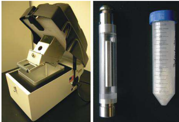
Figure 5.6 Tissue disruption using cryogenic grinding. A cryogenic mill (left), also known as freezer mill, can be used for the pulverization of hard tissue such as bone samples into fine powder prior to DNA extraction. During a grinding cycle, an impactor (right) moves back and forth, under a magnetic field, inside a grinding vial, grinding the sample to a fine powder. The grinding process is carried out at low temperatures (approximately -196^{\circ}\text{C} ), using liquid nitrogen to protect temperature-sensitive analytes such as DNA. (© Richard C. Li.)
