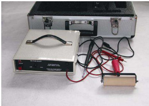
Figure 1.11 An electrostatic dust print lifting device can be utilized for processing impression evidence such as footprints and tire tracks. (© Richard C. Li.)
