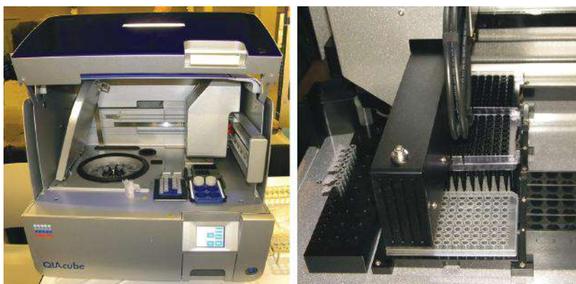
Figure 5.12 Automated bench-top DNA purification systems that enable the isolation of genomic DNA from a wide variety of forensic samples. A low-throughput sample-preparation system that can process up to 12 samples (left) and a low-to-medium throughput sample-preparation system (right). (© Richard C. Li.)
