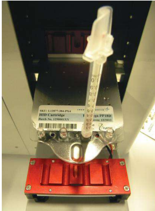
Figure 24.3 A rapid DNA instrument. A compact instrument that is designed to process swab samples and to produce DNA profiles within 2 h in the field. (© Richard C. Li.)
