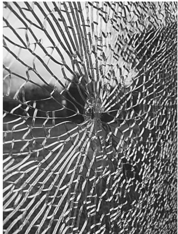
Figure 11.0.4 Penetrating hole in toughened glass caused by sharp stone.
