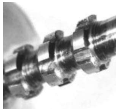
Figure 2.2.6 Part of a broach rifling cutter.
