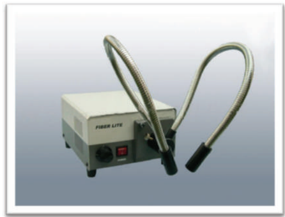
Figure 7.1.2 Single light source with fibre optic cables.
