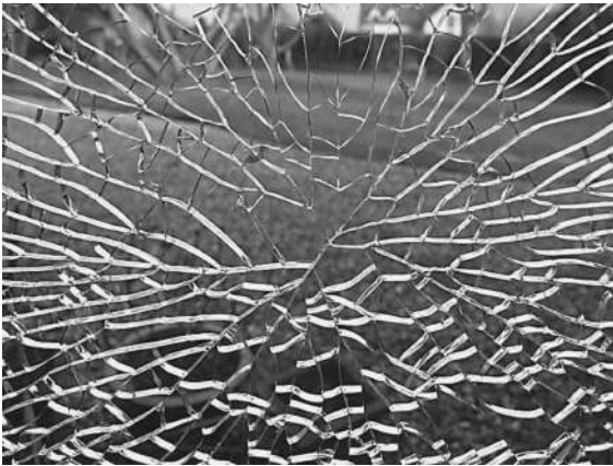
Figure 11.0.5 Non-penetrating damage caused by sharp stone.
