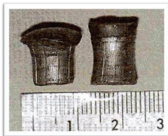
Figure 9.0.2 .357" Magnum bullets fired through a 6" and 2" barrel.
