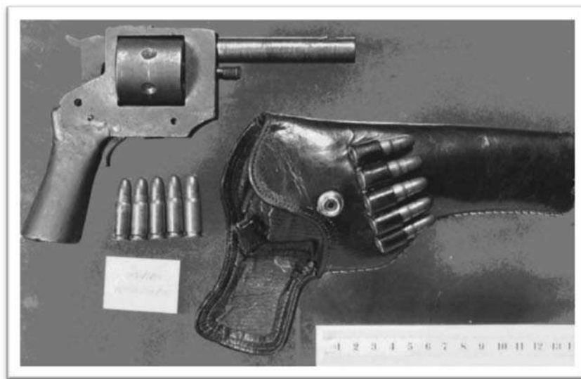
Figure 2.3.5 Home-made 7.62 × 25 mm calibre 'revolver' from the Far East.
