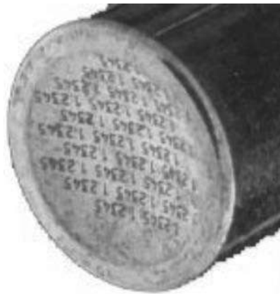
Figure 16.0.2 Laser-etched serial number on bullet.
