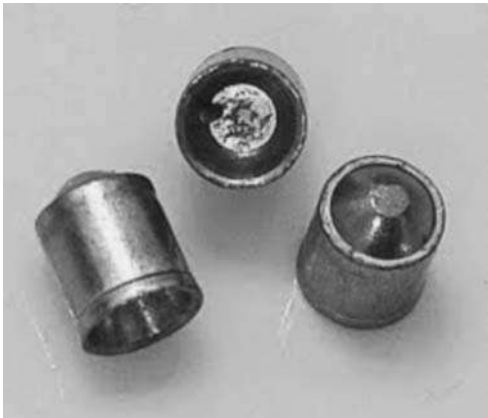
Figure 2.1.5 .20" (5 mm) Sheridan pellet.
