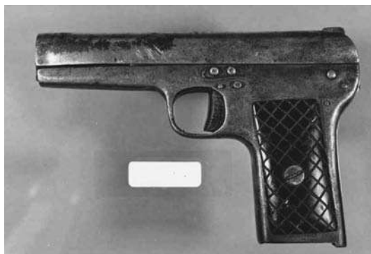
Figure 14.0.7 Home-made 7.62 × 25 mm pistol.
