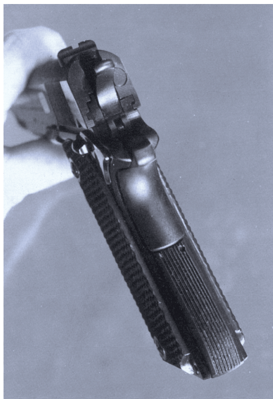
Figure 15.0.1 Colt 1911A1 pistol showing grooved back strap.
