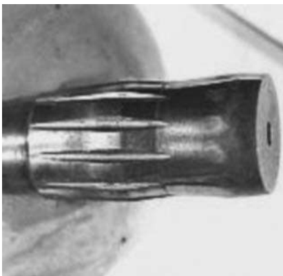
Figure 2.2.7 Button rifling tool.
