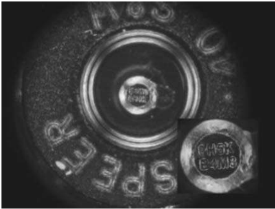
Figure 16.0.1 Firing pin impression from laser-etched serial number on firing pin.
