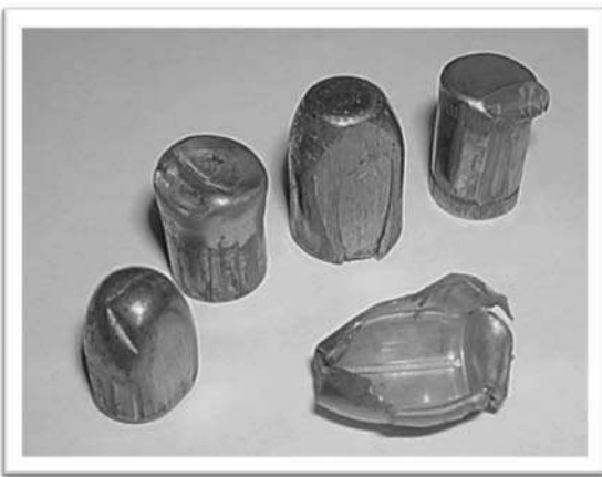
Figure 10.03 Typical appearance of jacketed bullets after having ricocheted from various surfaces.
