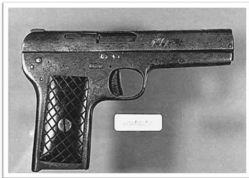
Figure 2.3.6 7.62 × 25 mm calibre home-made self-loading pistol.
