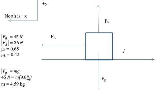
Notice here on the FBD that I just have *f*. I don't know if it is static OR kinetic yet. I know it acts to the south (right) because if this object remains at rest, the friction will need to counteract the applied force. I know that if the block moves due to the applied force, the velocity of the object will be to the north (left), therefore the kinetic friction will be to the south (right).
