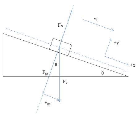
Side calcs  $\begin{vmatrix} F_{gx} \\ F_{gx} \end{vmatrix} = \begin{vmatrix} F_g \\ \sin \theta \end{vmatrix}$  $= mg \sin \theta$
