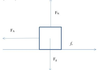
We are told the freezer remains at rest so the acceleration in the horizontal direction is zero. This is why we can presume the existence of the static frictional force going to the right otherwise the freezer would accelerate.
