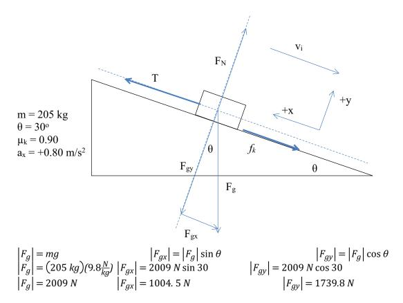
Since friction is in the problem, I first need to find the normal force so I can calculate  $f_k$
