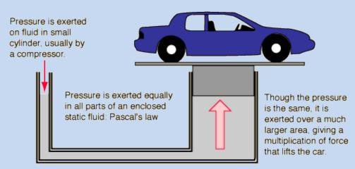
The force in the small cylinder must be exerted over a much larger distance. A small force exerted over a large distance is traded for a large force over a small distance.
