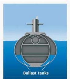
When a submarine is floating on the ocean's surface, its ballast tanks are filled mostly with air.
