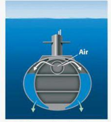
Vent holes are closed, and compressed air is pumped into the ballast tanks to force the water out, so the submarine rises.
