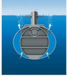
Vent holes on the ballast tanks are opened to allow the submarine to dive. Air escapes as the tanks fill with water.
