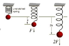
Provided the elastic limit of the spring is not exceeded (otherwise the spring breaks!), the
