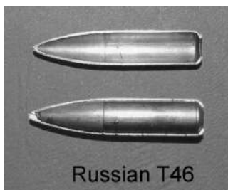
Figure 6.18 (See color insert.) Sectioned Russian 7.62 \times 54R Tracer bullet. The envelope is fitted with a relatively short lead alloy filling in its nose to achieve the appropriate weight, and a long, copper-coated, drawn steel pyrotechnic capsule in its extended rear section; an annular closure is visible from its base core end.
