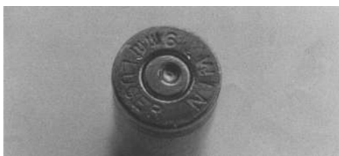
Figure 9.20 Unusual location of the ejector impact mark at 2 o'clock near the primer is characteristic in this instance of the use of a Polish Radom P35 9 mm self-loading pistol.
