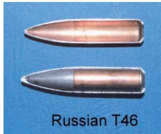
Figure 6.18 Sectioned Russian 7.62 × 54R Tracer bullet. The envelope is fitted with a relatively short lead alloy filling in its nose to achieve the appropriate weight, and a long, copper-coated, drawn steel pyrotechnic capsule in its extended rear section; an annular closure is visible from its base core end.
