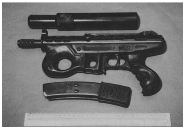
Figure 4.10 Unusual Yugoslav Agram 2000 submachine gun chambered for 9 × 19 mm ammunition was intercepted by port controls before arriving with other arms at its intended destination in a northwest city. The longer barrel that incorporates an integral silencer unit can be screwed in to replace the standard barrel.
