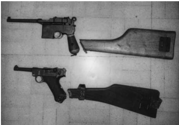
Figure 1.13 Top: 1896 Mauser 7.63 × 25 mm (.30) “Broomhandle” 10-shot self-loading pistol, with attachable, hollow holster stock. This early pistol used jacketed bullets and smokeless powder to generate muzzle velocities in the region of 1410 ft/s (430 m/s). A pistol of this type was used by young Winston Churchill in the last cavalry charge of the British Army in the Sudan. Bottom: Luger P’08 model 9 mm self-loading pistol with attachable shoulder stock usually fitted to the holster. Despite its age, this cartridge is still the foremost standard for use in pistols and submachine guns.
