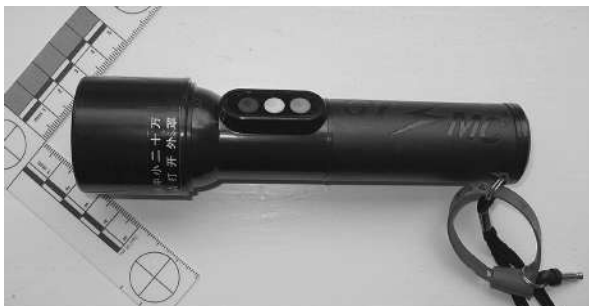
Figure 9.48 Chinese-manufactured powerful electronic stun gun in the form of a working flashlight. This particular device operates at an unusually high voltage. Care in handling is essential to avoid inadvertent exposure to a painful shock. It can be rendered safe for examination by first placing the exposed frontal electrodes in contact with a metal surface to “short out” any residual charge left after normal firing. Note additional flat anti-grab electrodes on side of head intended to prevent an adversary gaining possession of the weapon.
