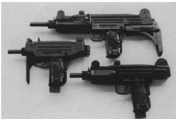
Figure 2.5 Semiautomatic variants of submachine guns were also caught by the 1988 legislation. Typified by the Israeli UZI range—standard arm with Mini and Micro variants. The diminutive “Micro” differs from the basic “L-shaped wrap-around open bolt” design of the other guns and fires from a closed breech. Here the bolt contains a tungsten filler to increase its mass without compromising its small size. However, the combination of small size and higher rate of fire makes the smaller models very difficult to control in automatic fire.
