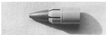
Figure 6.3 Remington .30-06 accelerator allows the firing of a .224 (5.56 mm) projectile from a popular deer rifle. The plastic sabot is discarded by the effects of air resistance a short distance from the muzzle. Manufacturers claim muzzle velocity of just in excess of 4000 ft/s (1220 m/s).
