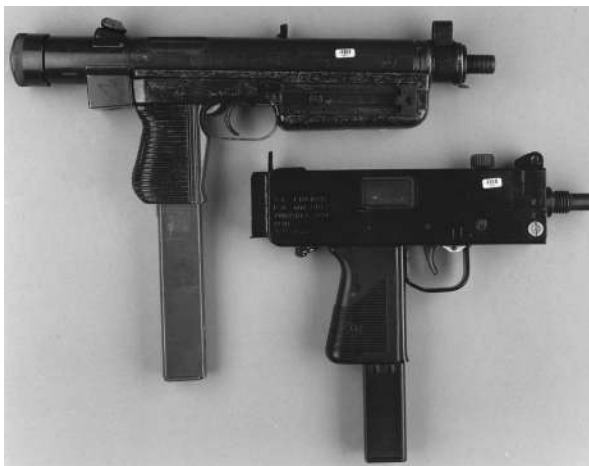
Figure 2.11 (See color insert.) Two examples of reactivated automatic weapons of the type seen frequently in criminal use in the U.K. in the past. Here shown is a Czech CZ-25 9 mm submachine gun (top) fitted with an unrifled replacement barrel, and a British assembled MAC-10-pattern gun (bottom) originally marketed as a 9 mm “target pistol,” which has been reactivated in a similar manner and threaded to allow the fitting of a silencer; the projecting lug at the rear end of its receiver allows the fitting of a rigid plastic shoulder stock. On a number of occasions Israeli subsonic ammunition best suited for use with moderated weapons was received with them.
