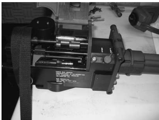
Figure 8.35 A 7.62 mm tank chain gun breech mounted on bench in firing room with one of a number of submitted barrels fitted to it. Firing was achieved manually on a single-shot basis into bullet collecting box using a wrench. Resulting test firings were then checked on the comparison microscope against the tracer bullet recovered from the clothing of the tank commander during the postmortem examination.
