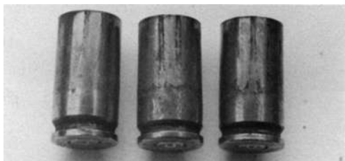
Figure 9.22 Distinctive chamber fluting marks left on 9 mm cartridge cases fired in a weapon of Heckler and Koch manufacture. Such distinctive effects greatly support or shorten the computer search for weapon type.
