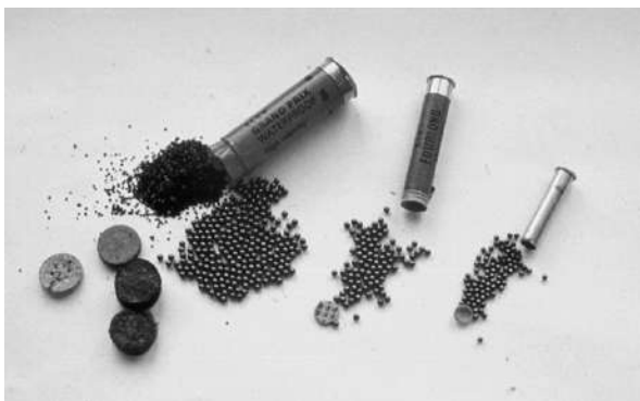
Figure 5.9 Disassembled 12-gauge, .410 in., and 9 mm rim-fire shotgun cartridges loaded with conventional shot loads and fiber wadding.
