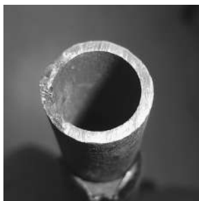
Figure 9.28 Typically rough muzzle end of crudely sawn-off shotgun likely to impart scratches on the exteriors of plastic cartridge wads. Marks of this nature found on wads recovered from a scene of shooting can be microscopically associated with a particular gun (see existing comparison microscope image Figure 9.29).
