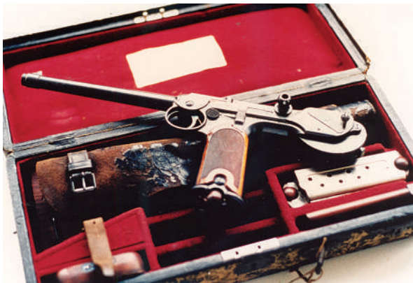
Figure 1.12 One of the first commercially successful self-loading pistols. The Borchardt recoil operated pistol of 1893 was chambered for a 7.65 mm smokeless powder cartridge employing a jacketed bullet, shown here with case and attachable shoulder stock. This pistol used an articulated link to provide the delayed opening of its locked breech similar to that used later for the Luger pistol.
