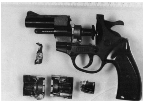
Figure 9.1 Light alloy blank revolvers that have had their blockages drilled out to allow their use with bulletted ammunition are surprisingly often capable of surviving many firings; shown here is an exception. A remote firing device and a polycarbonate safety shield should always be used when it is necessary to test fire such weapons.
