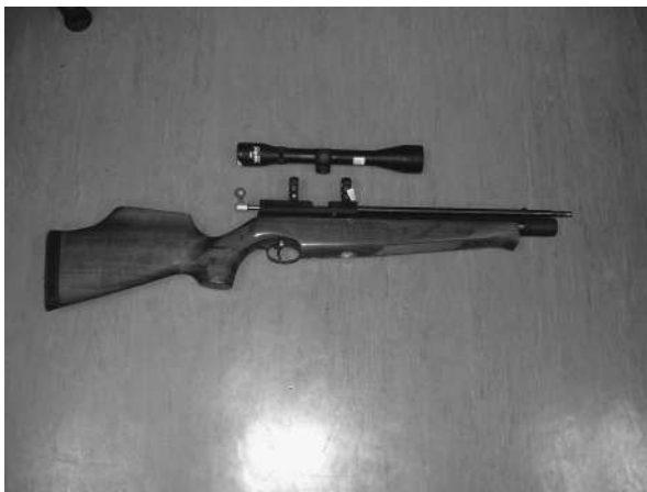
Figure 2.2 Modern precharged pneumatic air rifle. Air reservoir under barrel is charged using a diver's air bottle to provide up to about 80 full-power shots to be fired. Although the air release valve is usually set to provide missile kinetic energies just below 12 ft-lb (16 J), some models, which in Britain require a firearm certificate, are marketed to provide higher missile kinetic energies.
