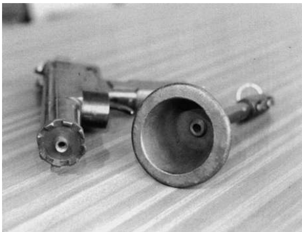
Figure 8.18 The varied geometry of the muzzle ends of humane killing devices, intended for use in abattoirs, can impart characteristic marks around the wound margins of human victims. Often such stunning devices will have been modified to better allow their use as a conventional firearm. In one case of suicide, the owner of a blank operated soft drinks can launching device had drilled out the offset chamber blockage to allow its use with a bulletted .22 rim-fire cartridge.
