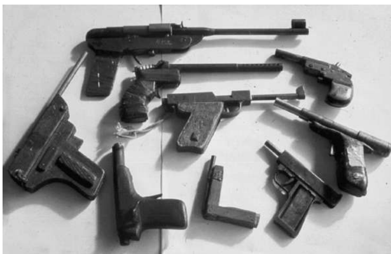
Figure 9.42 A few of the homemade guns (zip guns) received at the laboratory in casework submissions. The weapon shown at the top has been derived from an air weapon modified to allow the discharge of .22 rim-fire ammunition.
