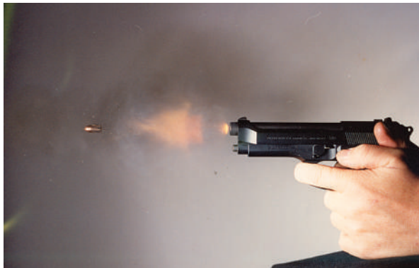
Figure 4.17 High-speed image of the firing of Beretta Model 92F 9 mm pistol. Fragments of unburnt propellant, capable of inflicting punctuate injuries to skin at short ranges, surround the bullet in flight. At this stage the slide has recoiled backward with the barrel to the point where the breech will begin to unlock, thus allowing the slide alone to move to its rearmost position to cause the extraction and ejection of the spent cartridge case, followed by the slide return under spring pressure to simultaneously strip and feed a fresh cartridge from its 15-shot magazine into the breech.
