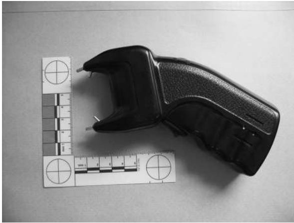
Figure 2.16 A relatively common type of electronic stun gun. The inner facing electrodes allow testing of weapon and visible discharge of spark between them.
