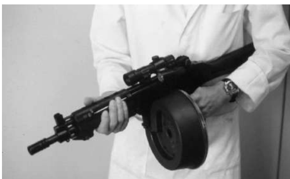
Figure 2.12 Post Firearms (Amendment) Act 1988 5.56 mm self-loading AR-18 design-based carbine fitted with 90-round drum magazine, marketed as a “target pistol.” The screw used for providing additional security for attaching the shoulder stock to its body was not supplied, and the title “Pistol” was inscribed upon its side, in an attempt to circumvent the ban on self-loading center-fire rifles and carbines.
