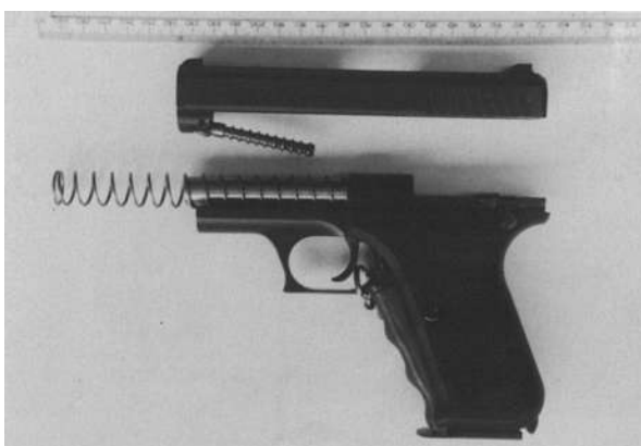
Figure 4.8 P7 pistol partially dismantled to reveal gas piston arrangement attached to the front end of the slide.
