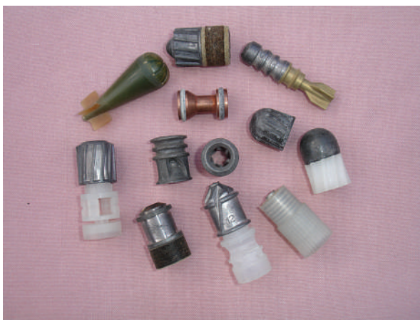
Figure 6.2 Examples of rifled and aerodynamically stabilized 12-gauge slugs. Missiles shown here include the classic German Brenneke rifled slug, the police issue Ferret fin-stabilized CS aerogel barricade-penetrating bullet, the old Blondeau slug with its artillery-style driving bands, the popular U.S. Foster rifled slug, and a subcaliber, fin-stabilized, discarding sabot bullet.
