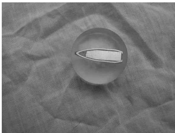
Figure 6.20 Sectioned Soviet M-43-pattern bullet used in the loading of 7.62 × 39 mm “PS Ball” ammunition. Truncated cone steel “penetrator” core of approximately 250 VPN (Vickers pyramid number) hardness held inside copper-coated steel jacket with a small amount of lead filler. This standard loading well outperformed the 5.56 × 45 mm lead-core loading when tested on the standard NATO battlefield helmet, eventually resulting in NATO adopting the heavier composite core Belgian SS109-pattern bullet.
