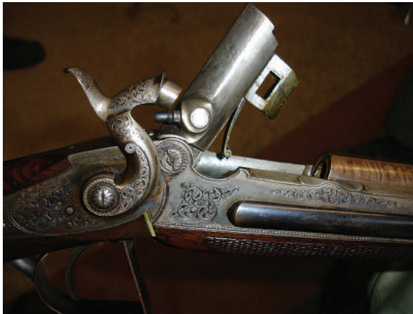
Figure 1.5 Antique capping breech-loading rifle typical of transitional mid-19th century firearms. The bullet and powder held in a consumable paper cartridge is inserted into the open breech section. After breech closure the flash generated by firing a standard percussion cap placed on the nipple causes discharge. Note the band pattern of Damascus twist barrel.
