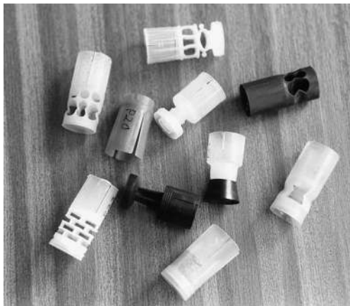
Figure 5.8 A few of the many different designs of plastic cup wads used in the loading of shotgun ammunition. The construction of the wadding has implications concerning close-range wound effects and the identification of the brand of cartridge used in an offense. Plastic cup wads for steel shot loadings are of much more robust construction, and in order to provide the necessary pellet capacity, they tend to dispense with the concertina-like shock-buffering section.
