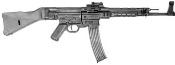
Figure 2.13 World War II German Sturmgeuer Stg .44 assault rifle, chambered for the intermediate power 7.92 × 33 mm Kurz cartridge, gave Kalashnikov the inspiration during combat he experienced on the Eastern Front, to design the AK47 and AKM assault rifles, chambered for a cartridge of similar power, the M.43 7.62 × 39 mm.
