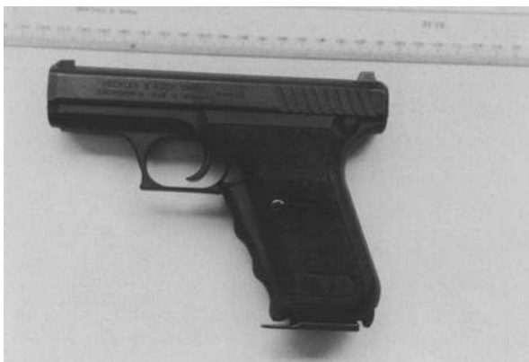
Figure 4.7 Heckler and Koch innovative gas retarded P7, 9 mm self-loading pistol that utilizes a squeeze-cocking/decocking device built into the grip.
