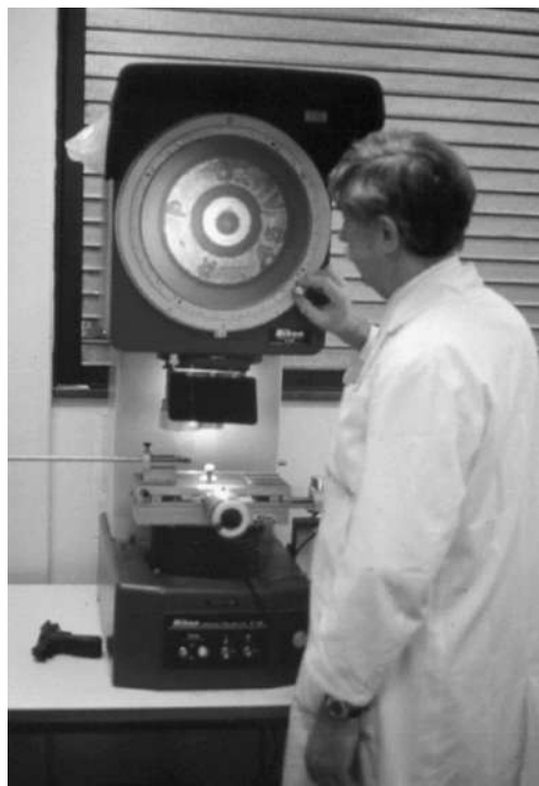
Figure 9.18 Examination and measuring of operational marks on cartridge cases and bullets using the profile projector allows the majority of the information for the FBI program computer search for weapon type to be accurately recorded.
