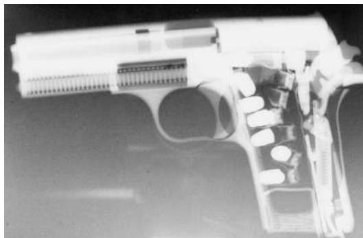
Figure 9.2 X-ray plate of seized-up fire-damaged pistol reveals that cartridges inside its magazine have been caused to explode by the heat. The picture confirms that it is now safe to attempt to free the pistol and disassemble it.
