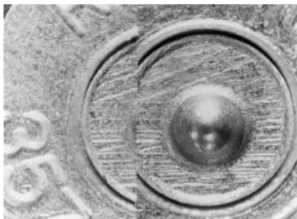
Figure 9.23 Match of .357 Magnum cartridge cases on comparison microscope. The marks in focus here have been imparted by the recoil face of the revolver. Correct choice of cartridge loading to best match that used in the crime is often essential, as electroplated finishes and differences in primer material hardness and pressure levels will affect the transfer of such marks.
