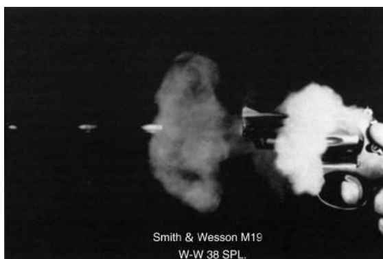
Figure 9.38 Three-channel high-speed photograph of firing of short-barreled S&W Model 19 revolver using Winchester .38 Special ammunition. The bright flash on the right is from the venting of high-pressure gases from the cylinder gap. Such an effect is likely to cause primer-generated GSR to be deposited on the hand, face, hair, and frontal clothing of the firer. The momentary opening of the breech of a self-loading pistol, pump-action/self-loading gun will also likely cause similar transfer effects to take place.
