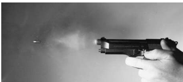
Figure 4.17 (See color insert.) High-speed image of the firing of Beretta Model 92F 9 mm pistol. Fragments of unburnt propellant, capable of inflicting punctuate injuries to skin at short ranges, surround the bullet in flight. At this stage the slide has recoiled backward with the barrel to the point where the breech will begin to unlock, thus allowing the slide alone to move to its rearmost position to cause the extraction and ejection of the spent cartridge case, followed by the slide return under spring pressure to simultaneously strip and feed a fresh cartridge from its 15-shot magazine into the breech.
