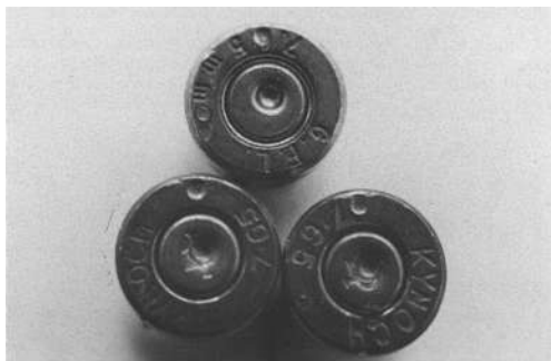
Figure 9.21 Marks left at 12 o'clock positions on the cartridge cases indicate a self-loading pistol with a loaded chamber indicator pin, in this instance a Walther PPK.
