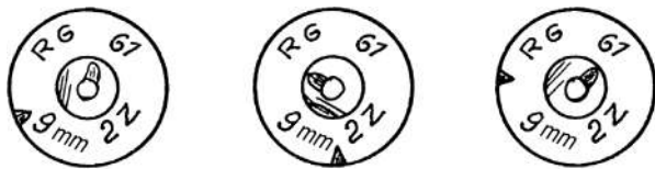
Figure 9.17 Fired cartridge cases showing the locations of operational markings. The headstamps indicate that all of the British Service 9 × 19 mm 2Z type cartridges were manufactured at the Radway Green Ordnance Plant in Cheshire in the year 1961.
