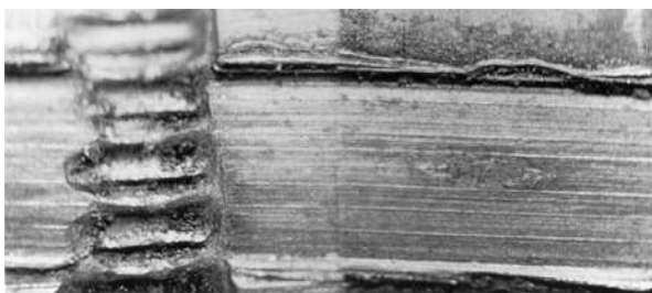
Figure 9.26 Match of an old .380 British Service revolver bullet recovered from the head of female victim against test fire from S&W revolver recovered from underneath floorboards in millionaire’s gun room. Earlier at the postmortem I had formed a tentative conclusion after examining the bullet that it had probably been fired from a S&W revolver using WWII Canadian manufactured Service ammunition. After I found several cartridges of this same type hidden in a gun cabinet, the police SOCOs took the room apart and recovered the murder weapon.
