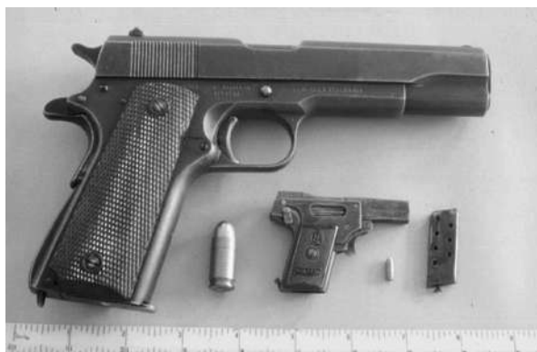
Figure 4.4 Firearms do not have to be large to be lethal. Shown here is the old U.S. Army-issue 1911A1 45 self-loading pistol next to the diminutive Kolibri 2.7 mm self-loading pistol of 1914. Ballistics claimed for the 2.7 mm round: 198–213 m/s and 4 J (650–680 ft/s and 3 ft-lb).
