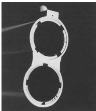
Figure 5.6 Modern screw-in choke tubes are a convenient alternative to conventionally choke bored barrels. Rifled choke tube units are also available to increase the accuracy of single slug loadings. The four shallow square cut recesses at the end of the choke tubes allow the use of a special tool for their removal or fitting. The narrow grooves cut in the end signify the degree of choke boring. A single slot in the upper tube signifies “full choke,” while the three in the lower tube signify “modified choke.” To guard against possible damage to the female threaded end of the barrel, it is usual for suppliers to warn against firing the gun without a choke tube fitted.
