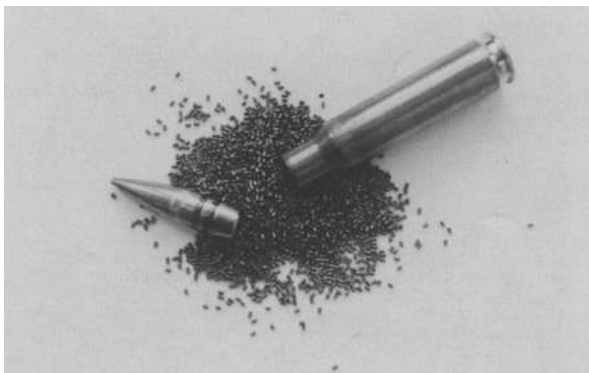
Figure 5.1 The cartridge loading at the heart of the firearm heat engine. N.A.T.O. 7.62 × 51 mm rifle and machine gun loading. However, not all of the energy released by the burning of the powder charge is imparted to the projectile.
