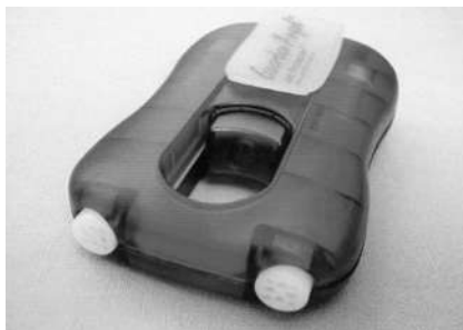
Figure 9.47 Swiss-manufactured Guardian Angel self-defense device. This two-shot device uses the impulse generated by the discharge of a special blank cartridge to project the capsaicin-based agent through multiholed nozzles as a dispersed pattern over an effective range of between 1.5 and 13 ft (0.5–4 m).
