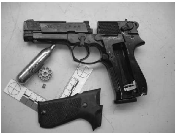
Figure 2.9 Walther CP88 carbon dioxide-powered pistol closely resembling a 9 mm self-loading pistol, with eight-shot rotary magazine into which standard waisted air gun pellets are loaded. This low-powered pistol is treated in the same way as a conventional air pistol in Great Britain.
