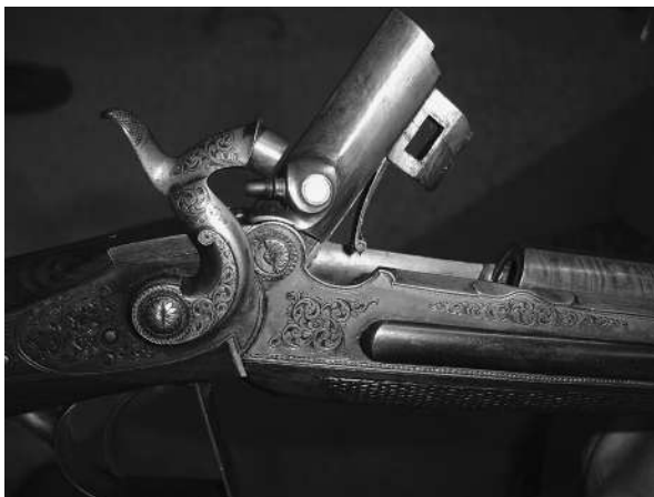
Figure 1.5 (See color insert.) Antique capping breech-loading rifle typical of transitional mid-19th century firearms. The bullet and powder held in a consumable paper cartridge is inserted into the open breech section. After breech closure the flash generated by firing a standard percussion cap placed on the nipple causes discharge. Note the band pattern of Damascus twist barrel.
