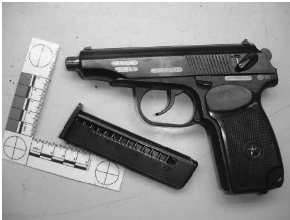
Figure 2.17 One of a number of Russian-manufactured “Baikal” self-loading pistols originally marketed for use with 9 mm PA blank and tear-gas cartridges, closely resembling a Soviet “Makarov” 9 mm service pistol, illegally smuggled into the U.K. from one of the Baltic states recently admitted into the EC. Here the barrel, along with its original partial blockages, has been drilled out and fitted with a steel liner chambered for popular 380/9 mm Short ammunition; Russian “Wolf” brand bulletted ammunition supplied with it; the muzzle end of the extended barrel has also been threaded to allow the fitting of a silencer. The original serial numbers and some of its other markings have also been machined away, leaving only the Russian Izhevsk proof marks for the year 2005. Although the barrel of this particular pistol has been crudely rifled with six-groove left-hand twist, other examples have exhibited a variety of unusual rifling patterns.
