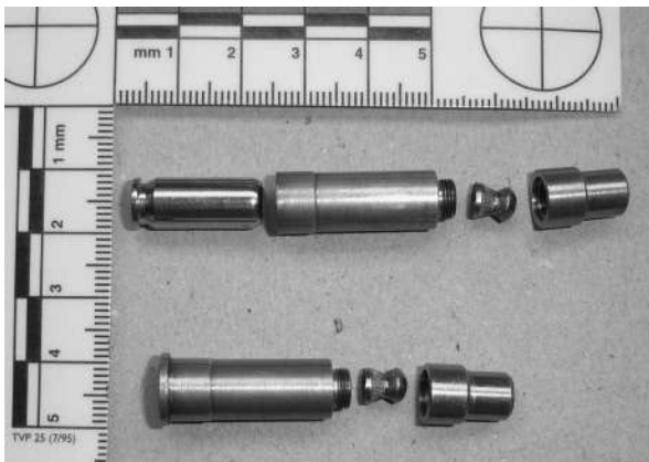
Figure 2.14 Modified tandem air cartridge (TAC) with .22 pellet and 9 mm PA center-fire blank cartridge shown with standard “TAC” below. Magnum pellets (30 gr/1.94 g) can also be used to form improvised ammunition with these marginally modified self-loading air pistols.
