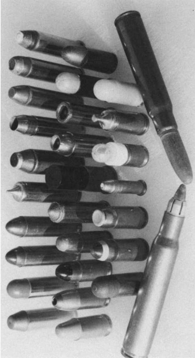
Figure 6.15 An assortment of special and exotic cartridge loadings. Starting at the left side of the back row: .38 Special tungsten polymer bullet loading; MBA 38 Special Short-Stop; Israeli .357 Magnum CBAP armor piercing; Israeli CBX Cavity-Wounding; French SFM THV; Velet .44 Special Mercury filling; PMC 38 Special Tubular; National 357 Magnum Tracer; Velet 357 Magnum explosive; Bingham 38 Special explosive; KTW 9 mm armor piercing; Geco 9 mm Action 3; Israeli 9 mm CBAP; Geco 9 mm Effect Nose; 38 Special Quad; Speer Target 44 Plastic primer-powered training; Federal 10 mm Hydra-Shock; 38 Special Scorpion; SNC-FX 38 Marker; Geco 9 mm Action Safety; TEC 9 mm Frangible; Israeli 9 mm CBAP; Glaser 9 mm Safety Slug; Bingham 22 LR Devastator explosive; SNC-FX 9 mm Simunition; SFM 9 mm THV; Geco 9 mm Plastik Training; Remington .30-06 Accelerator; 7.92 mm Mauser wooden bullet rifle blank.
