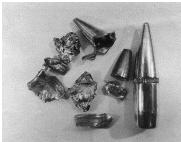
Figure 7.15 The composite form and the design of the current NATO 5.56 mm bullet loading frequently leads to missile blow-up effects at close ranges. The truncated cone steel penetrator from the core is shown in the center right of the field.
