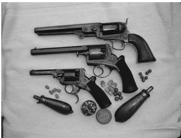
Figure 1.4 (See color insert.) Three of the author's antique percussion, muzzle-loading revolvers. Top: Colt 1851 .36 in. "Navy" originally bought for British Service use during the Crimean War period. This is one of a number refinished at the Pimlico facility on return from this war, resulting in loss of naval battle scene on cylinder. Center: Robert Adams' "double-action only" 5-shot 54-bore revolver of period did not secure the government contract, although a number of officers purchased them for their own use. Bottom: William Tranter's Third Model double-trigger 120-bore revolver of 1856 offered accurate rapid fire. Pulling back the outer trigger with the middle finger cocked the hammer and rotated the cylinder, while a second short and light pull to the inner trigger caused it to fire. Nostalgia and Spaghetti Westerns ensured the manufacture of reproduction arms predominantly in Italy, particularly those models used in the U.S. Civil War period.
