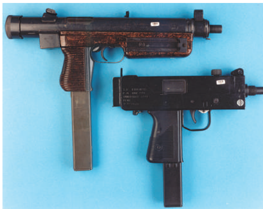
Figure 2.11 Two examples of reactivated automatic weapons of the type seen frequently in criminal use in the U.K. in the past. Here shown is a Czech CZ-25 9 mm submachine gun (top) fitted with an unrifled replacement barrel, and a British assembled MAC-10-pattern gun (bottom) originally marketed as a 9 mm "target pistol," which has been reactivated in a similar manner and threaded to allow the fitting of a silencer; the projecting lug at the rear end of its receiver allows the fitting of a rigid plastic shoulder stock. On a number of occasions Israeli subsonic ammunition best suited for use with moderated weapons was received with them.
