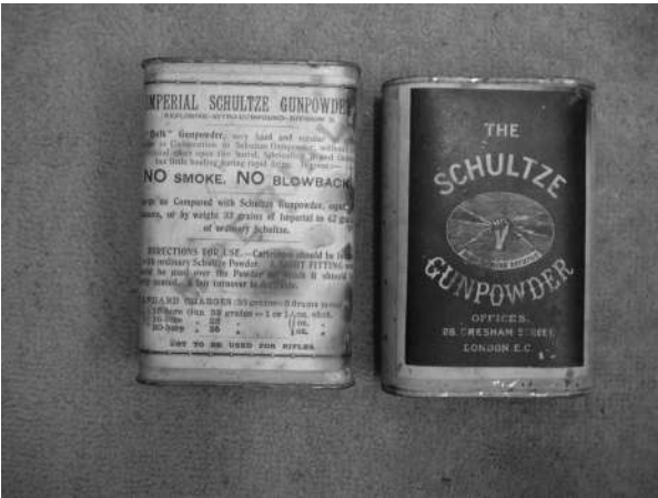
Figure 1.10 An early example of a dense loading smokeless powder, in this case “Imperial Shultze.” Instruction on container indicate that 33 gr (~2.14 g) serve in place of a 3 dram/82 gr/5.3 g charge of black powder in a 12-gauge shotgun cartridge loading. Accidents occurred in early years when some people persisted in using their old dram volume measuring devices with the new dense powders.
