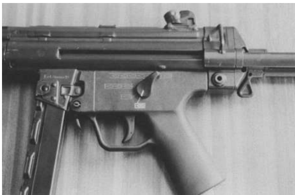
Figure 4.12 Heckler and Koch trigger grouping with fire selector to suit all tastes. Pictorial markings, intended to minimize any language barrier, indicate safe, single-shot, three-round burst or full-automatic modes of operation. Optional groupings calling up burst-fire operation involving a different number of cartridges are available to order.
