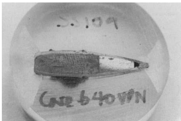
Figure 6.17 Microsection of NATO SS109 5.56 mm bullet showing truncated cone-shaped hard steel core in front of the plain lead alloy filling.
