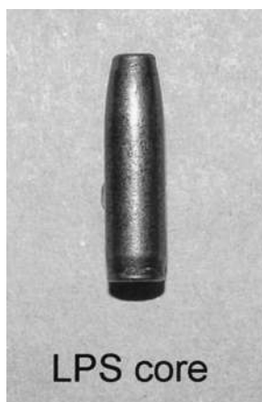
Figure 7.9 Steel bullet core from Russian 7.62 × 54R LPS Light Ball recovered from abdomen of British TV news reporter shot outside Basra by Iraqis firing a truck-mounted PK machine gun while pursuing the reporters' sport-utility vehicle. The bullet shed its jacket to strike his lower back sideways on after passing through the rear of his vehicle (Gulf War II).
