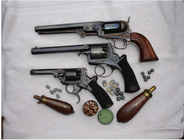
Figure 1.4 Three of the author's antique percussion, muzzle-loading revolvers. Top: Colt 1851 .36 in. "Navy" originally bought for British Service use during the Crimean War period. This is one of a number refinished at the Pimlico facility on return from this war, resulting in loss of naval battle scene on cylinder. Center: Robert Adams' "double-action only" 5-shot 54-bore revolver of period did not secure the government contract, although a number of officers purchased them for their own use. Bottom: William Tranter's Third Model double-trigger 120-bore revolver of 1856 offered accurate rapid fire. Pulling back the outer trigger with the middle finger cocked the hammer and rotated the cylinder, while a second short and light pull to the inner trigger caused it to fire. Nostalgia and Spaghetti Westerns ensured the manufacture of reproduction arms predominantly in Italy, particularly those models used in the U.S. Civil War period.
