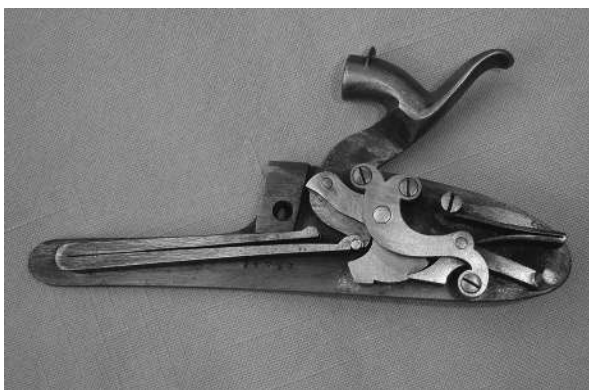
Figure 4.1 Hammer shotgun lock showing the “v”-spring fully compressed as the hammer has been pulled back to the full cock position, causing the tip of the sear to become engaged in the shallow full-cock notch (bent) of the tumbler.
