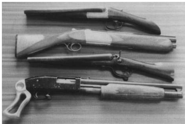
Figure 2.1 Sawn-off shotguns received at the laboratory in casework submissions. Derived from double-barreled side-by-side English-pattern gun, double-barreled over-and-under gun of the type commonly used in clay pigeon shooting, Jones action double-barreled side-by-side hammer gun manufactured in the 1860–1870 period, and an American Mossberg pump-action gun.
