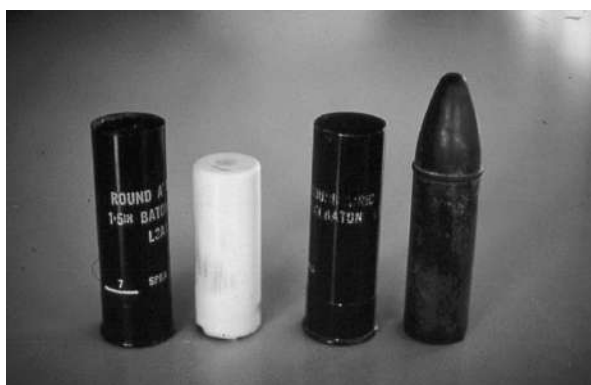
Figure 6.14 Riot control baton rounds, 1.5 in./37 mm. The original shaped black rubber bullet was replaced by an ivory colored polyurethane plastic bullet in an attempt at reducing the incidence of fatalities in service use in Northern Ireland.
