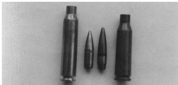
Figure 6.16 NATO 5.56 \times 45 mm versus the Soviet 5.45 \times 39 mm loading. The use of a slightly smaller caliber and a steel core bullet enhances the ballistic shape of the Soviet loading as well as conferring a significant improvement in its ability to defeat light screening cover. The relatively new NATO SS109 bullet configuration, which has replaced the original plain lead core loading, includes a part steel core and an increased weight to achieve similar enhanced downrange performance and penetration.
