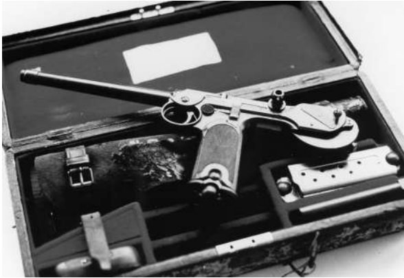
Figure 1.12 (See color insert.) One of the first commercially successful self-loading pistols. The Borchardt recoil operated pistol of 1893 was chambered for a 7.65 mm smokeless powder cartridge employing a jacketed bullet, shown here with case and attachable shoulder stock. This pistol used an articulated link to provide the delayed opening of its locked breech similar to that used later for the Luger pistol.
