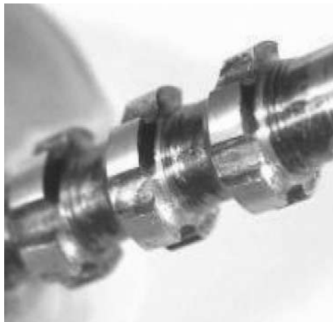
Figure 4.6 Broach rifling cutter.
