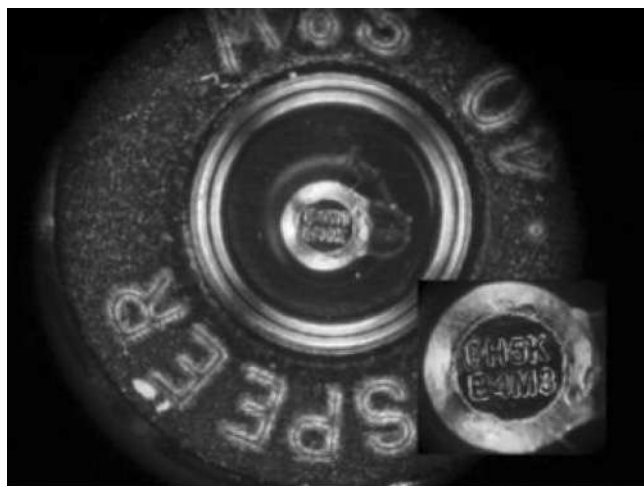
Figure 8.3 Firing pin impression with laser-etched serial number.
