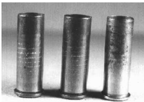
Figure 4.23 Annular ring chamber marks on fired cartridge case.
