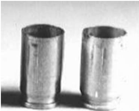
Figure 4.20 Scoop chamber marks on fired cartridge case.
