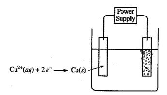
3. An external direct-current power supply is connected to two platinum electrodes immersed in a beaker containing 1.0 M CuSO<sub>4</sub>(aq) at 25°C, as shown in the diagram above. As the cell operates, copper metal is deposited onto one electrode and O<sub>2</sub>(g) is produced at the other electrode. The two reduction half-reactions for the overall reaction that occurs in the cell are shown in the table below.
