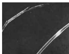
Silk Fiber: left fiber: fracture, right fiber: crossover indentation.
