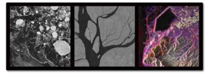
**LEFT**: The ERS-1 satellite sends out wavelengths about 5.7 cm long (C-band). This image shows sea ice breaking off the shores of Alaska. **CENTER**: The JERS satellite uses wavelengths about 20 cm in length (L-band). This is an image of the Amazon River in Brazil. **RIGHT**: This is a radar image acquired from the Space Shuttle. It also used awavelengthin the L-band of the microwave spectrum. Here we see a computerenhanced radarimage of some mountains on the edge of Salt Lake City, Utah.
