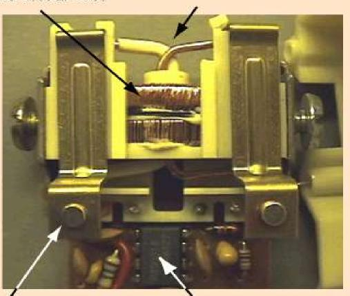
Contacts break both "hot" and neutral in case of fault current
