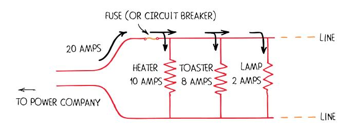
In practice, the lines in your home are not perfect conductors. With the large current used to operate a vacuum cleaner, the connecting wires do warm up. But for most cases, the resistance of the lines can be neglected.
