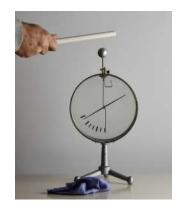
**b.** Explain the behavior of the electroscope needle (1) when the charged rod touches the electroscope and (2) then when it is brought closer to the charged electroscope without touching.
