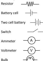
Note: Circuits could be drawn differently than these as long as the essential elements are included correctly.
