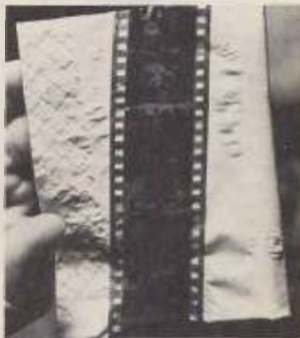
Careful removal of all excess wetting agent from the base side of films with lint-free wiping cloths is one sure way to avoid formation of scum.
