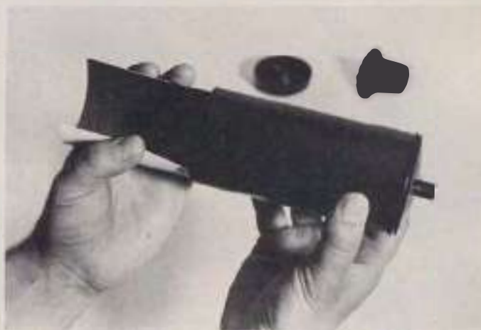
Loading the Cibachrome drum is easy, but you must insert the paper in total darkness.
