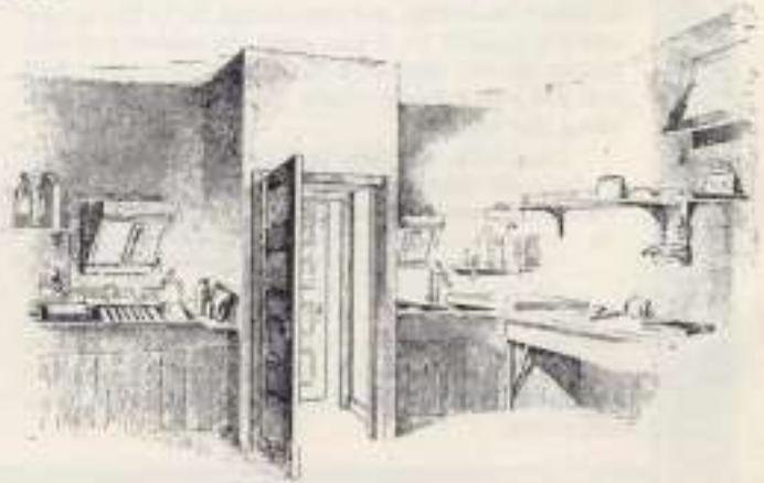
A Typical Darkroom of the 1880s. Papers were contact printed and produced the same size print as the negative. They were exposed in the frames mounted to the wall on either side of the door.
