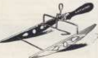
Allderige's Developing Racker. Agitation during development was as important in the 1880s as it is today.
