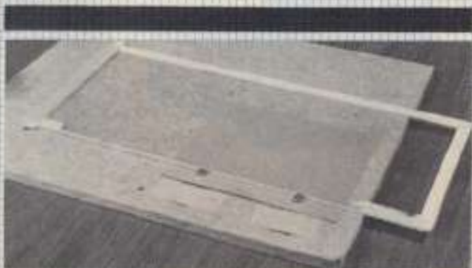
Photo E: Completed registration board with glass pressure plate taped all around for safety.
