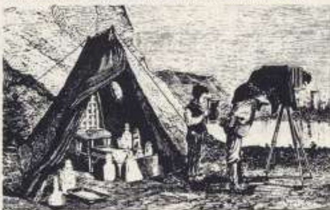
A Portable Darkroom of the 1860s. The darkroom of this period had to be set up close to the camera so the plate could be coated, loaded into the camera, and returned to the darkroom for development after the exposure and before the emulsion dried.
