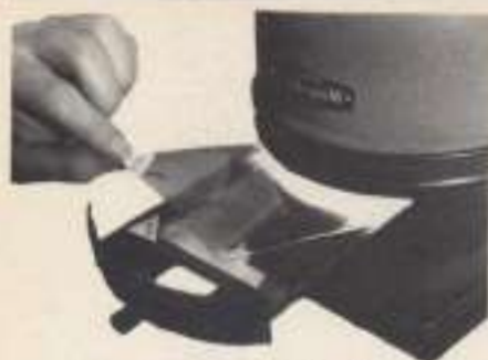
With virtually any standard enlarger, you can inexpensively control the color of your printing light by using acetate filters in the filter drawer.
