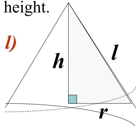
Notice that the height (h) (altitude), the radius and the slant height create a right triangle.
