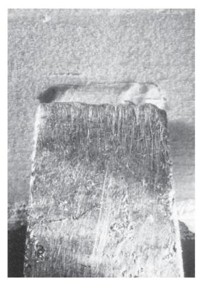
A comparison of a tool mark with a suspect screwdriver. Note how the presence of nicks and breaks on the tool's edge helps individualize the tool to the mark.
