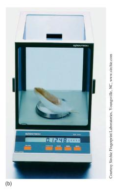
(a) Top-loading balance. (b) Single-pan analytical balance.
