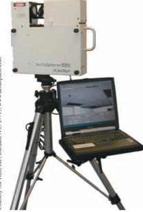
A computer-controlled scanner has both a high-resolution, professional digital camera and a long-range laser rangefinder. The tripodmounted device rotates a full 360 degrees, taking dozens of photographs and measuring millions of individual points. Photographic and laser data from multiple scan locations are combined to produce 3D models of the scene.
