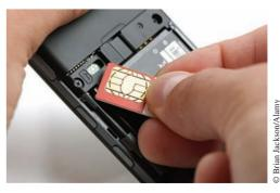
**FIGURE 19–4** A SIM inserted in a cell phone.
