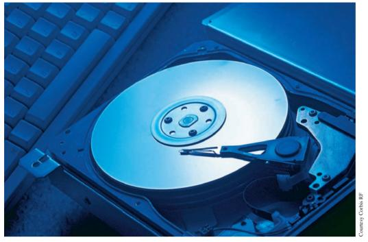
An inside view of the platter and read/write head of a hard disk drive.
