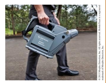
*Hardened* MobileTrace®, a portable ion mobility spectrometer used to rapidly detect and tentatively identify trace quantities of explosives.
