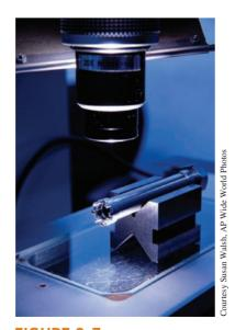
FIGURE 8–7 A segment of a broach cutter.
