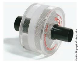
Vacuum sweeper attachment, constructed of clear plastic in two pieces that are joined by a threaded joint. A metal screen is mounted in one half to support a filter paper to collect debris. The unit attaches to the hose of the vacuum sweeper. After a designated area of the crime scene is vacuumed, the filter paper is removed and retained for laboratory examination.
