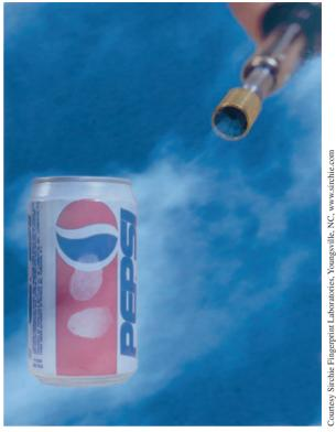
**FIGURE 6–15** Superglue fuming a nonporous metallic surface in the search for latent fingerprints.
