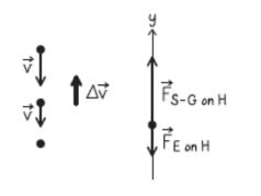
downward gravitational force  $\vec{F}_{E \text{ on } H}$ . The force diagram is the same for all points of the motion diagram because the acceleration is constant. On the force diagram the arrow for  $\vec{F}_{S-G \text{ on } H}$  must be longer to match the motion diagram, which shows the velocity change arrow pointing up.
