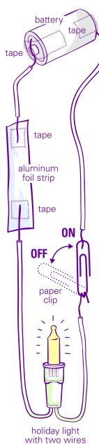
Tape one end of each stripped wire to each end of the battery, so the bare wire touches the center of each end of the battery.
