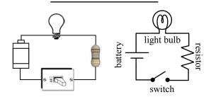
The diagram on the right is a faster way of drawing the circuit on the left. (Notice the direction of the battery, which is important)
