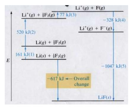
7. Write the reactions for each step, the  $\Delta H$  for each step, and then add to give the net reaction and net  $\Delta H$  as on the previous page.
