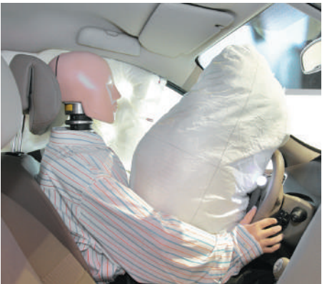
FIGURE 3.7 An air bag stops a crash test dummy during a collision.
