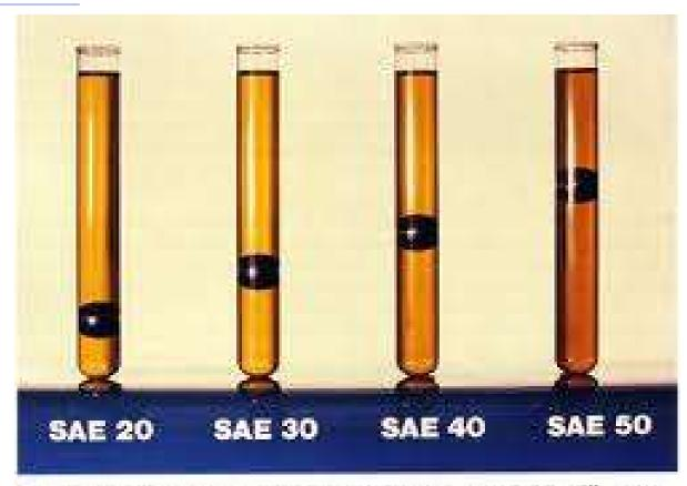
Sized balls of equal weight dropped into test tubes filled with motor oils fell at different rates. Their rate of fell depends on the viscosity of the oil. The ball travelling through the light SAE 20 oil has travelled farthoot, while the ball in the heavy SAE 50 has travelled least.
