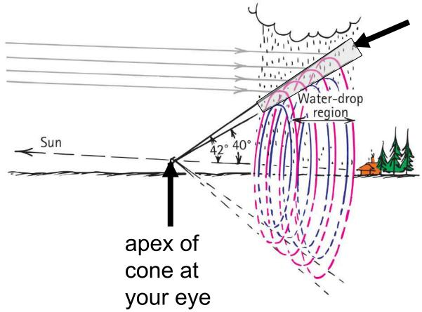
The thicker the region containing water drops, the thicker the conical edge you look through, and the more vivid the rainbow. The cone has different layers with drops that disperse red to your eye on the outside, orange beneath the red, yellow beneath the orange, and so on, all the way to violet on the inner conical surface.
