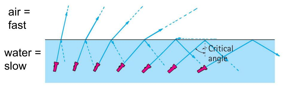
As angle of incidence in water increases.... ....angle of refraction increases,
