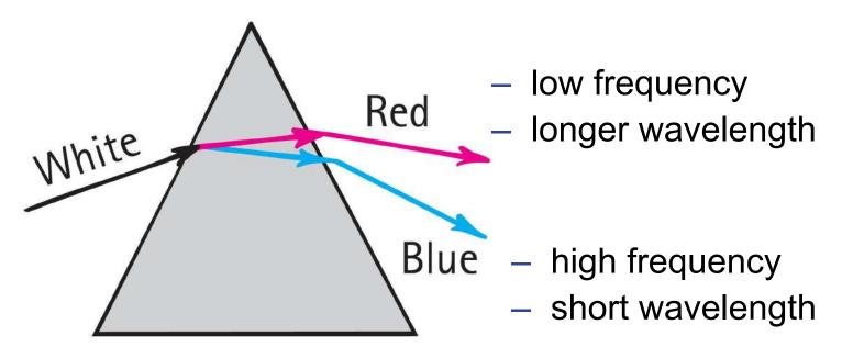
Components of white light are dispersed (spread out) in a prism.
