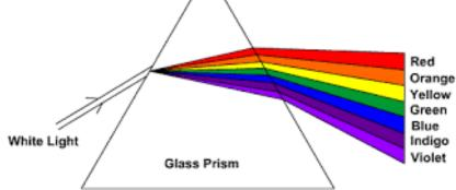
Refraction leaving the glass spreads them even more because sides of the prism are not parallel.
