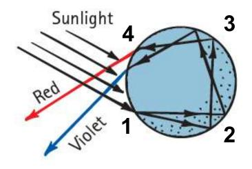
Bow is reversed in color (due to extra internal reflection).
