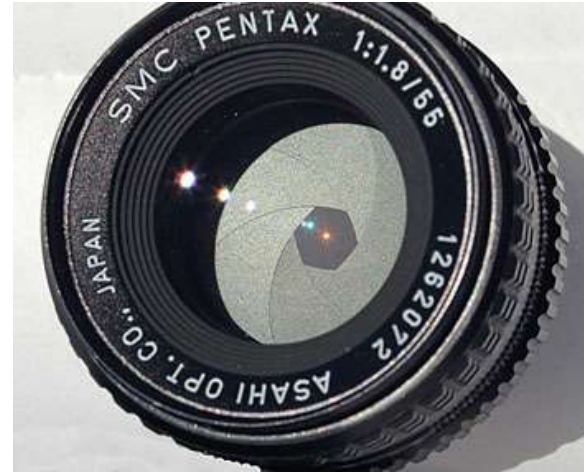
Camera Diaphragm The plates in the iris diaphragm fold in on each other to shrink the aperture and expand out to make it wider.
