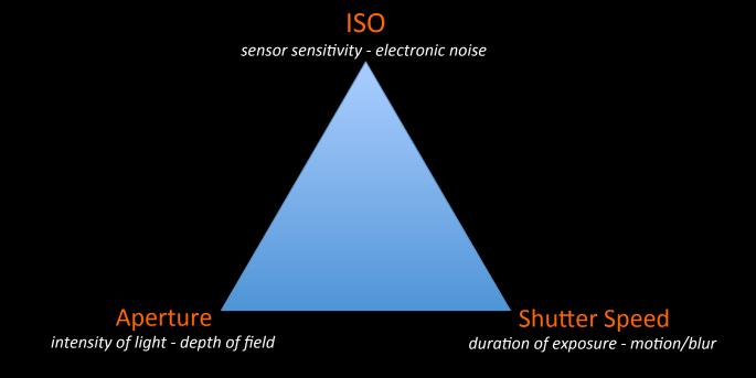
Exposure is solely controlled by the shutter speed, aperture, and ISO. Making creative decisions on what aperture, shutter speed, and ISO to use is necessary before firing your shutter.
