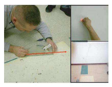
**Figure 8.39** The use of a laser protractor for stringing a scene. The protractor is aligned to the directional angle and set at the indicated impact angle. The end of the string is then attached to the point where the laser dot appears.
