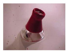
**Figure 8.23** A photographer's loupe in use to measure a stain.
