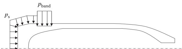
FIGURE 4.16 Load conditions for an M1 highly explosive projectile.
