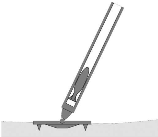
FIGURE 6.2 Baseplate-mounted trench mortar cannon.
