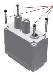
Carefully remove case screws with a small jeweler's phillips screwdriver
