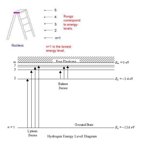
Above is the energy diagram of a hydrogen atom.
